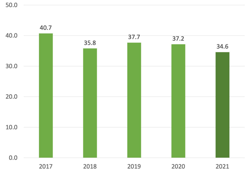
Criteria Air Emissions from Refineries (VOC, NOx, CO, SO2 & PM10) Metric Tonnes / Million barrels of Throughput*
