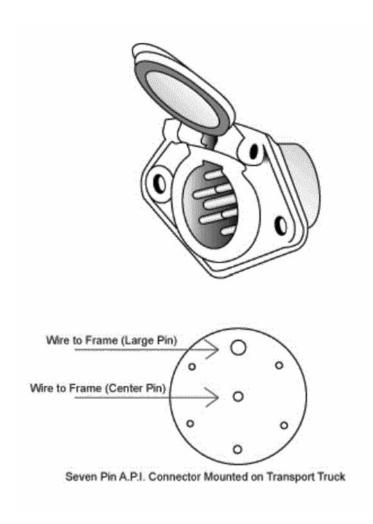
Both the Top Pin and Center Pin must be wired directly to the frame of the trailer by a wire approximately 4 to 5 inches long.
