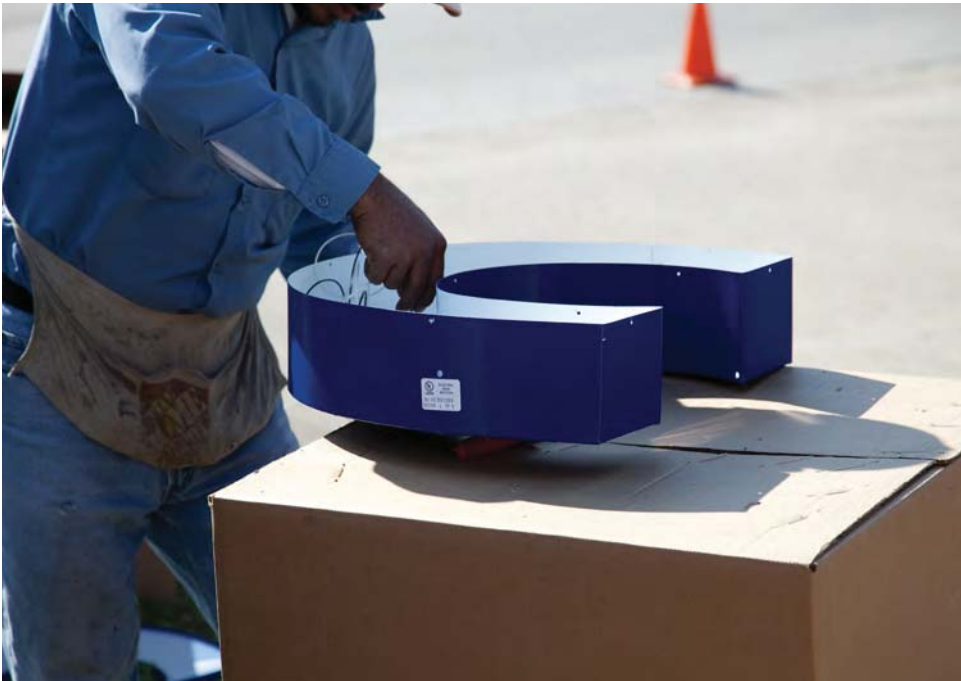
Preparing the secondary white CITGO channel letters. Note the blue sides of the channel letter.
